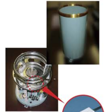
Anti-freezing of the rain gauges
