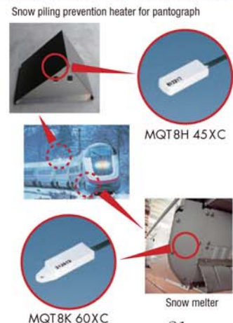
Countermeasures against snow for the bullet train
